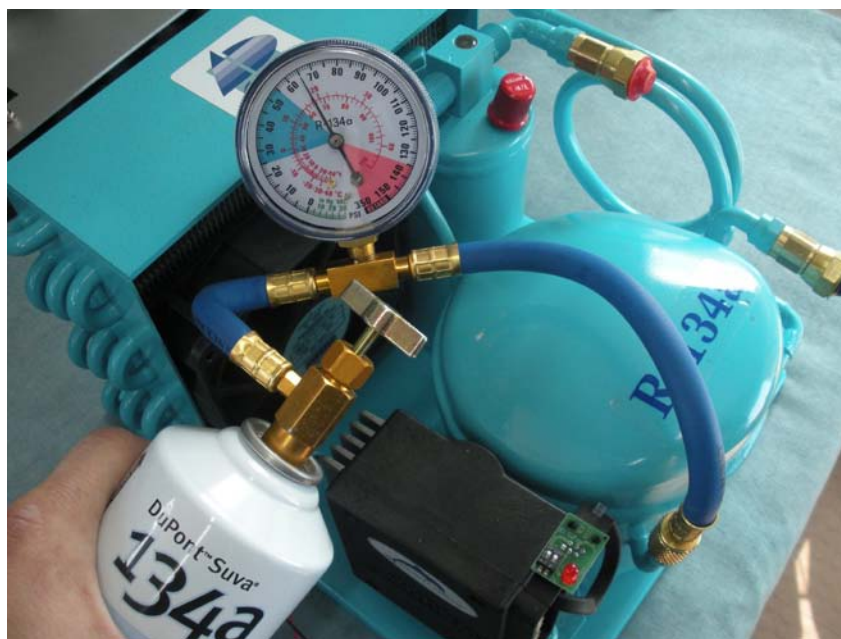
Figure 19: Freon System Recharge Connection
