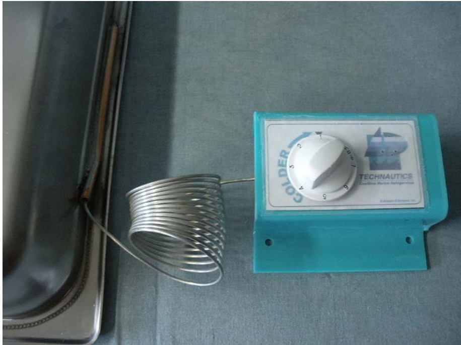
Figure 4: Thermostat Sensing Line Location
