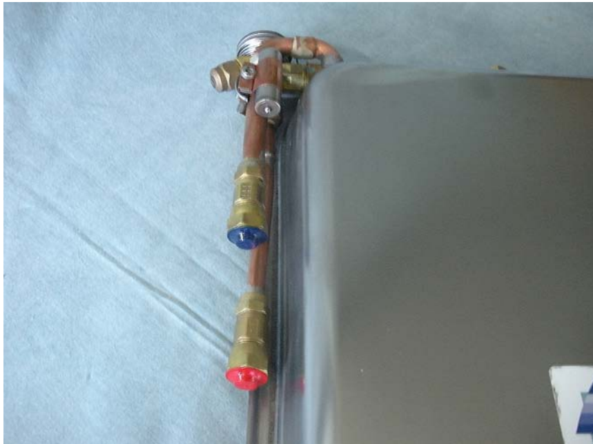
Figure 13: Cold Plate Refrigerant Connection Lines
