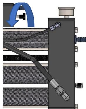
5. Close the reset valve (lever in vertical position).
