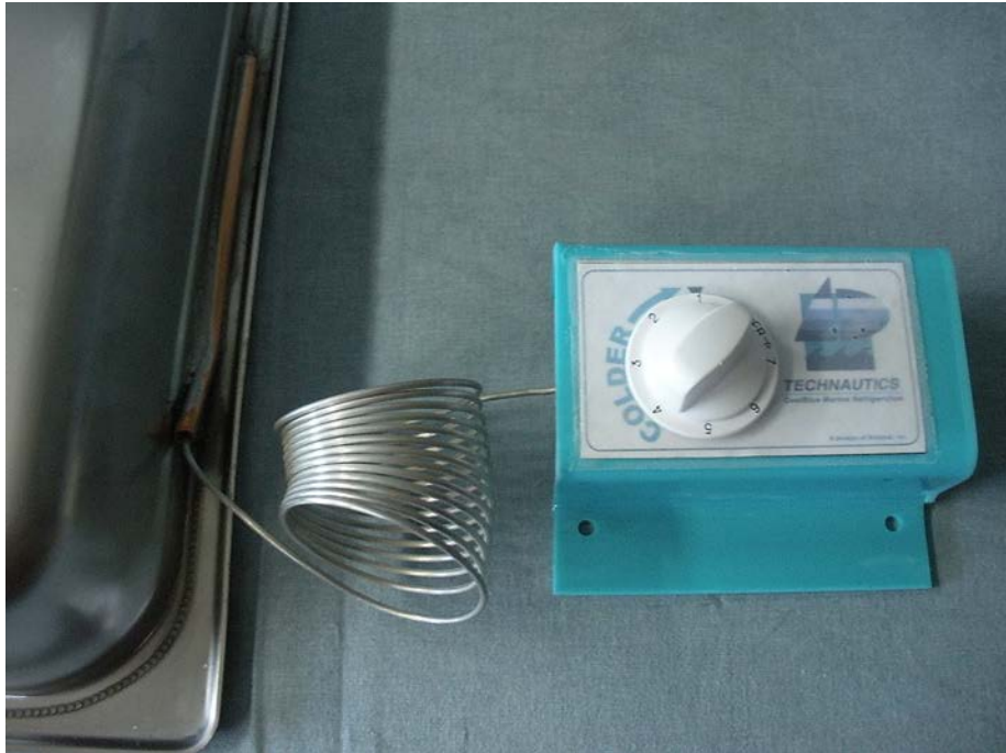
Figure 5: Thermostat Sensing Line Location
