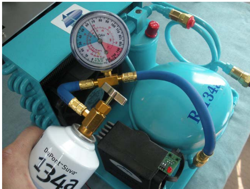
Figure 24: Compressor Recharge Port for Adding Freon
