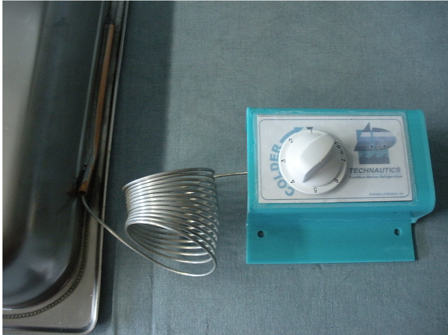
Figure 5: Thermostat Sensing Line Location
